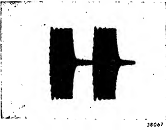
Fig. 144. Oscillogram of the alternating voltage across a normally-oscillating circuit as a function of time, the anode supply being periodically interrupted.
