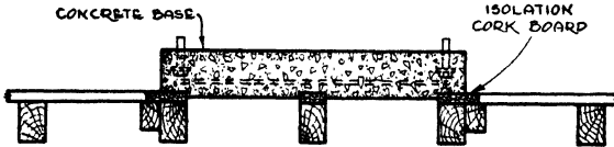
Fig. 6. Foundation—Mill Type Floor Construction
