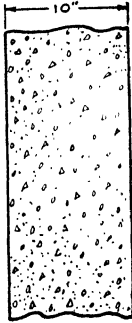
Fig. 3. Section through a Plain 10-inch Concrete Wall
