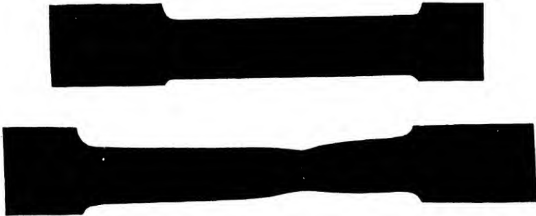
Fig. 21. Test Piece before and after Being Broken by Tension
