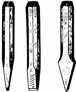
FIG. 255. TYPES OF CHISELS (1) Round-nose (2) Flat (3) Cross-cut
