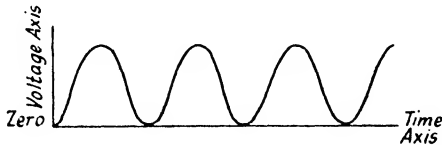
FIG. 62. DIRECT CURRENT OBTAINED BY USING APPARATUS SHOWN IN FIG. 61
