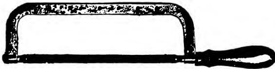
FIG. 268. HACK SAW, WITH ADJUSTABLE FRAME
