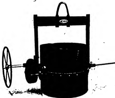
FIG. 159. CRANE LADLE WITH WORM AND BEVEL GEARING
