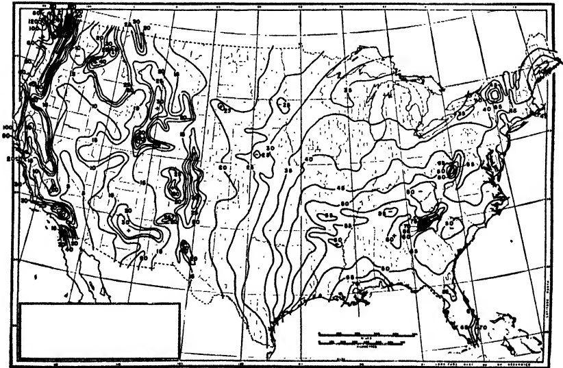
FIG. 6-30. Annual precipitation equaled or exceeded 25 per cent of the time. (After Lackey.)
