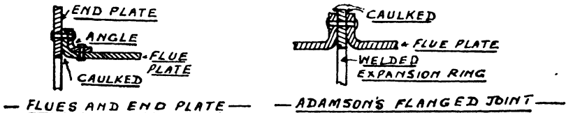
FIG. 124.—Boiler Flue Joints and Connections.
