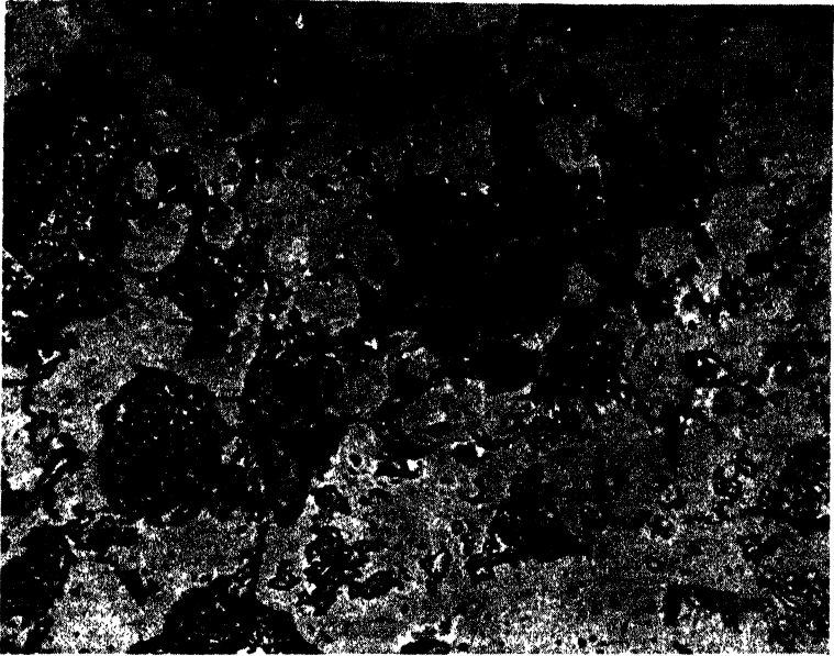
Figure 33. Typical rounded grains of free CaO in clinker. Water etch, \times 1000 . (Ward)
