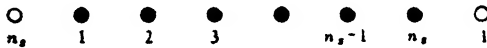
Fig. 15. Group of r_s sites (full circles); the two end sites are repeated at the opposite ends (open circles) to eliminate end effects.
