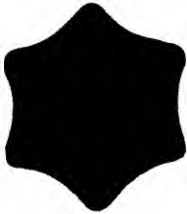
FIG. IX-10.—Fluted ingot for making cannon tube. This form allows what Howe calls "the virtual expansion of the outer walls" (see page 246), without cracking those walls. It also allows the interior to expand without cracking the exterior. Finally, it avoids weakness due to crystal junctions (see Fig. VIII-22).
