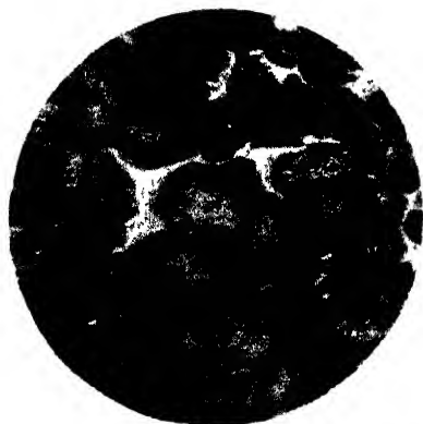
FIG. XI-19.—Micrograph of gray cast iron containing 2.6 per cent of silicon. Etched in 1 per cent picral. 500 \times . The only constituents showing are graphite, ferrite, and pearlite. ( Charles A. Turner, Jr. )
