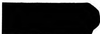
FIG. IX-13.—Shape of ends of rolled metal when the inside is the hotter.
