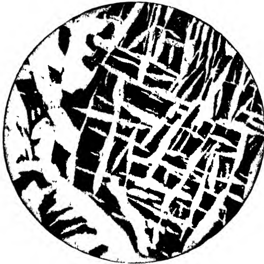
FIG. IX-1.—Crystals of cast steel, magnified 100 diameters, showing large size ( Courtesy of James M. Camp. )
