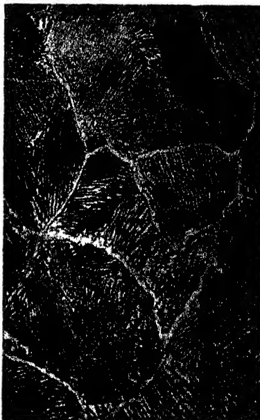
FIG. XII-6.—Crystals of cementite surrounding crystals of pearlite. 500X. (Hanemann and Schrader.)
