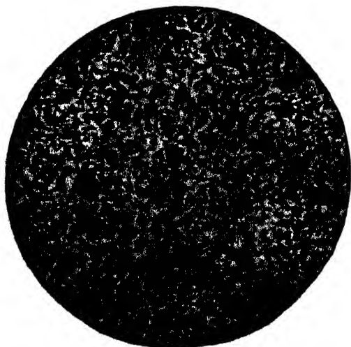
FIG. IX-8b.—Effect of finishing temperature. Crystals of steel magnified 100 diameters. The steel, like that in Fig. IX-8a, was subjected to mechanical working while hot, but the finishing temperature was low. (Courtesy of James M. Camp.)
