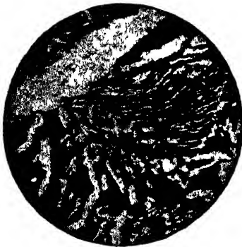
FIG. XII-2.—Big cementite crystal in pearlite. 250 \times . Polished in relief.
