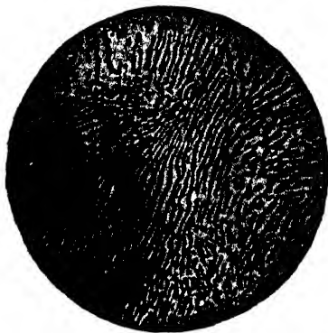
FIG. XI-12.—Pearlite eutectoid of iron and carbon. ( F. Osmond. )
