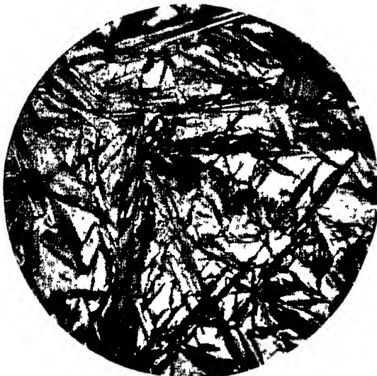
FIG. XIII-22 —Martensitic structure. 1500 X. (Micrograph by F F Lucas.)
