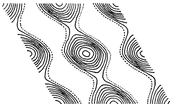
FIG. 1. Tobacco necrosis protein. Patterson-Fourier projection along the c axis. The vector distribution shown here is of the simplest form: the peaks correspond only to vectors between the large molecules and provide no evidence of internal structure.
