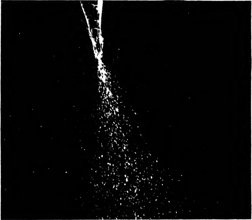
FIG. 183.—Blowing last drop from pipette. Pipette was allowed to drain, then last drop was blown out with moderate force. (After Johansson and Ferris.)
