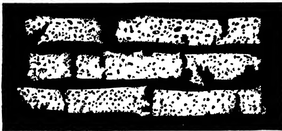
FIG 202—Strips of filter paper showing disintegrated areas due to bacterial attack. (After Omelianski; from Lipman's "Bacteria in Relation to Country Life," The Macmillan Company, New York)
