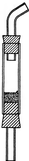
FIG. 176.—A modification of the Petri sand filter adopted by the American Public Health Association, 1909.
