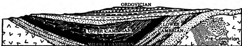
62. Diagrammatic section showing structural relations and divisions of Cambrian rocks in Wales. Important unconformities occur below and above the Cambrian System. In places, however, Ordovician strata lie parallel on Upper Cambrian beds.
