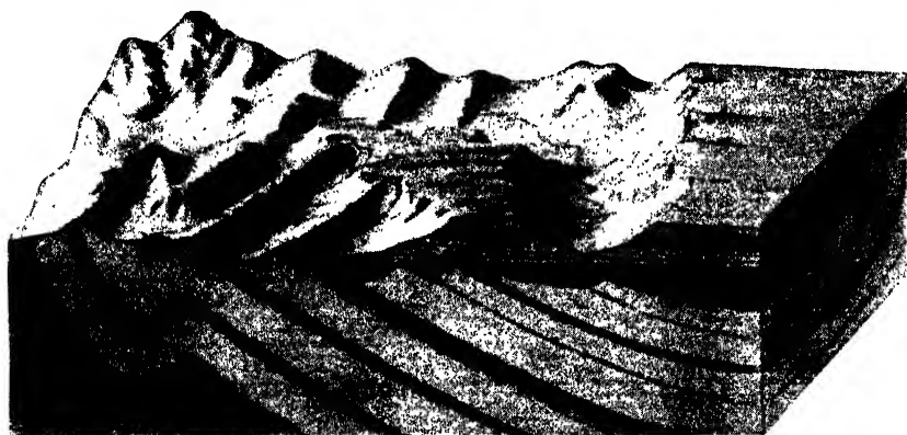
20. Geologic dating of crustal deformation. The diagram, which represents part of the eastern border of the Rocky Mountains, shows two sequences of stratified rocks having discordant structure. The tilted and folded beds were truncated by erosion before deposition of the horizontal overlying series. Hard rocks of the folded series make hogbacks, and weak strata form monoclinal valleys. The deformed and eroded rocks were buried beneath younger deposits and then subsequently exhumed partly. The geologic date of the folding must be later than the youngest deformed stratum and older than the lowermost horizontal deposit.
