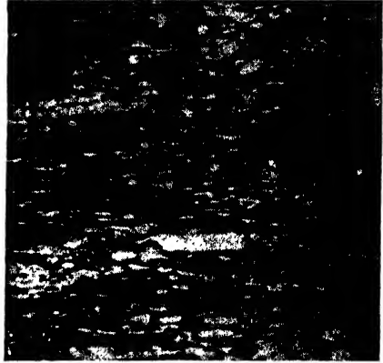
150. Very thin slice of coal cut at right angles to bedding. Viewed by transmitted light, only a small part of a thin section of coal is opaque. The light-colored constituents are various kinds of plant debris. Much magnified. (R. Thiessen, Illinois Geol. Survey. )
