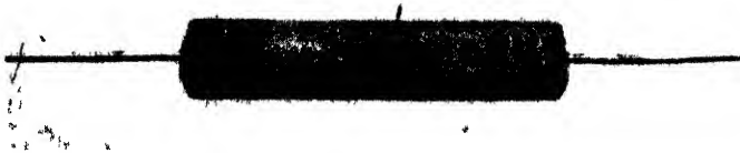
FIG. 35.—Photograph of a resistor of the “composition” instead of wire-wound type. This resistor will only dissipate one watt. They are made in values of from a few ohms to millions of ohms.
