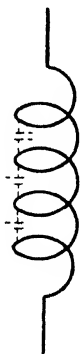
FIG. 195.—Distributed capacitance exists between the turns of a coil. Some resistance is also introduced by the wire composing the coil.
