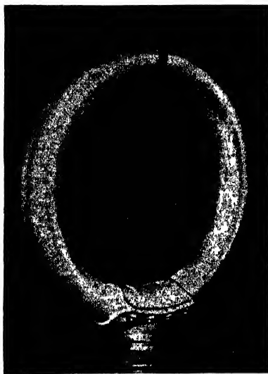
FIG. 214.—A shielded loop antenna such as used in an aircraft radio compass. The metallic shield is broken at the top as shown to prevent the shield from acting as a short-circuited turn. (Courtesy of Bell Telephone Laboratories.)
