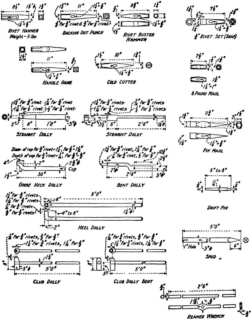
FIG. 7-23. Tools for Steel Erection. (Courtesy American Bridge Co.)
