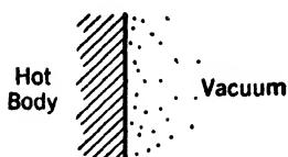
FIG. 1. Thermionic emission of electrons.
