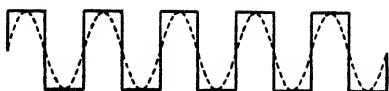
Fig. 2.2—Rectangular waveform with a superimposed sine wave (dotted) of the same repetition frequency
