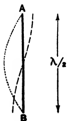
Fig. 19.1—The current and voltage distribution in a half-wave aerial are shown here
