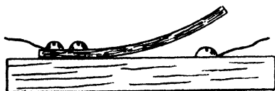
FIG. 11 SWITCHES FOR THE TELEPHONE PROJECT
