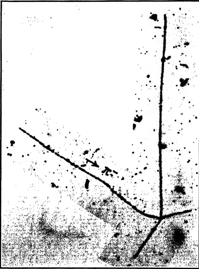
Fig. 14-2. Collision of a fast \pi meson with a nucleus. The meson is of negative sign. Three charged particles are emitted. (After C. F. Powell, Reports on Progress in Physics, 13 (1950). The Physical Society, London; "Mesons," Plate II.)
