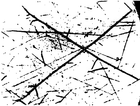
Fig. 13-1. Cloud-chamber tracks of two independent fission fragments. (Courtesy of C. C. and T. Lauritsen.)
