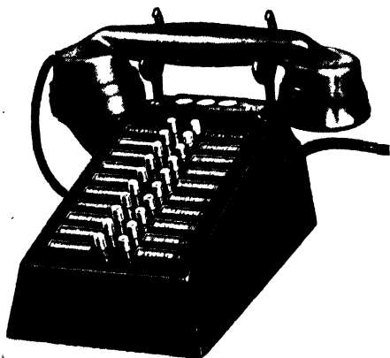
FIG. 101.—INTER-COMMUNICATION SUBSTATION TELEPHONE FITTED WITH BUTTONS FOR CALLING THREE MASTER STATIONS AND SEVENTEEN SUBSTATIONS.
