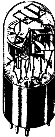
Fig. 4-19, below. Sketch of the functioning elements of the Phasitron tube and a simplified schematic diagram of the circuits to which they are connected. Above and below the electron disk is the deflection system. The deflector grids consist of 36 wires every third one being connected, making three grids each having 12 wires. The voltages indicated in this and the next figure are typical of slightly different operating conditions.
