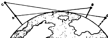
Fig. 5-14. The line of sight is shown between two antennas at A and B. If the antenna A were raised to position C, the line of sight would be extended to D.
