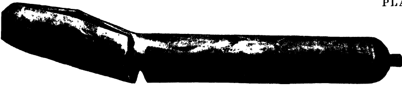
Cylinder U.H. 12. Normalized at 830 to 850° C. Nominal Thickness 0.26". Pressure at Elastic Limit—297 Atmospheres. Bursting Pressure 504 Atmospheres.
