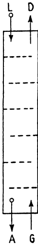
FIG. 114. Diagrammatic representation of column for separation of carbon monoxide from coke-oven gas.
