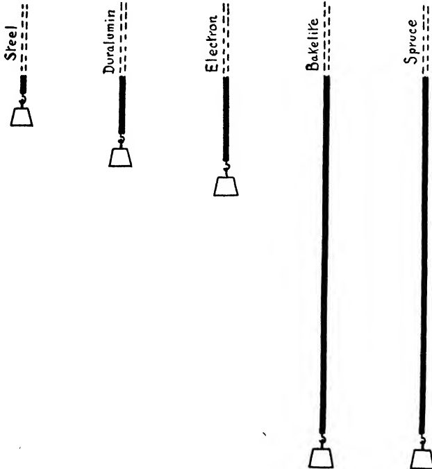
FIG. 19. HOW THE MATERIALS STRETCH UNDER LOAD (WITHIN THE ELASTIC LIMIT)
