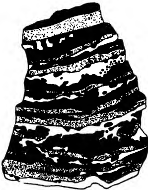
FIG. 107.—Banded sulphur-bearing rocks from Sicily; black, sulphur; dotted, limestone; white, calcite. (From Stutzer, Die Nicht-Erze .)
