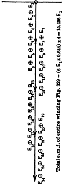
FIG. 331. Topographic vector diagrams of voltages across the four series groups in winding of Fig. 329.
