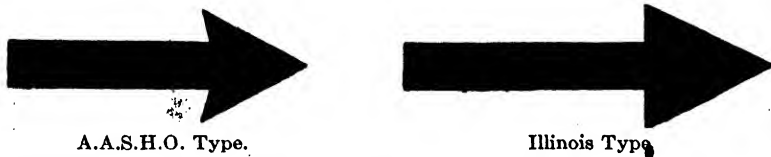
FIG. 20-11.—Arrows. The A.A.S.H.O. arrow has been enlarged 12\frac{1}{2} percent to give it the same shaft width as the Illinois arrow but even when enlarged its effectiveness is only about 70 percent compared with the other.
