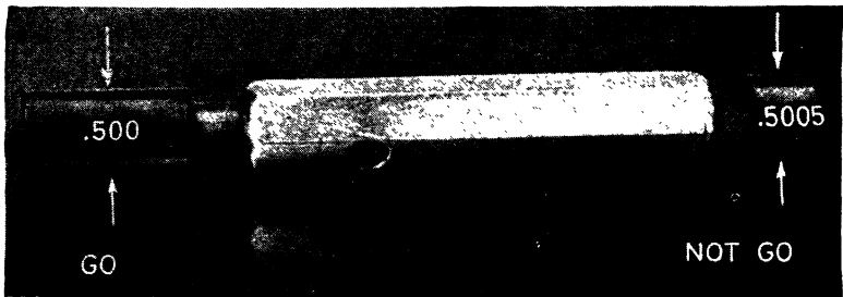
FIG. 60.—Taper lock cylindrical plug gage showing go and no-go plugs and handle with drift hole. (Courtesy of U.S. Office of Education.)
