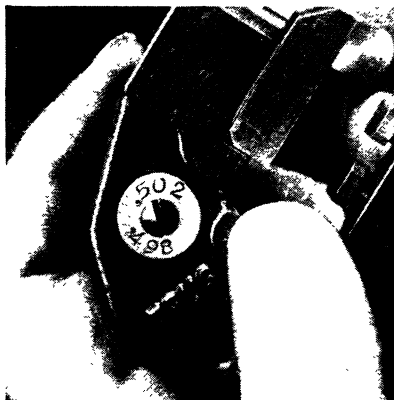
FIG. 59.—Marking disk of snap gage. (Courtesy of U.S. Office of Education.)
