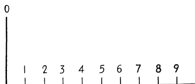
FIG. 10.—The inch divided according to the decimal system.
