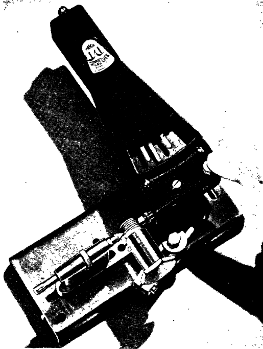
FIG. 86.—Thread checking fixture.
