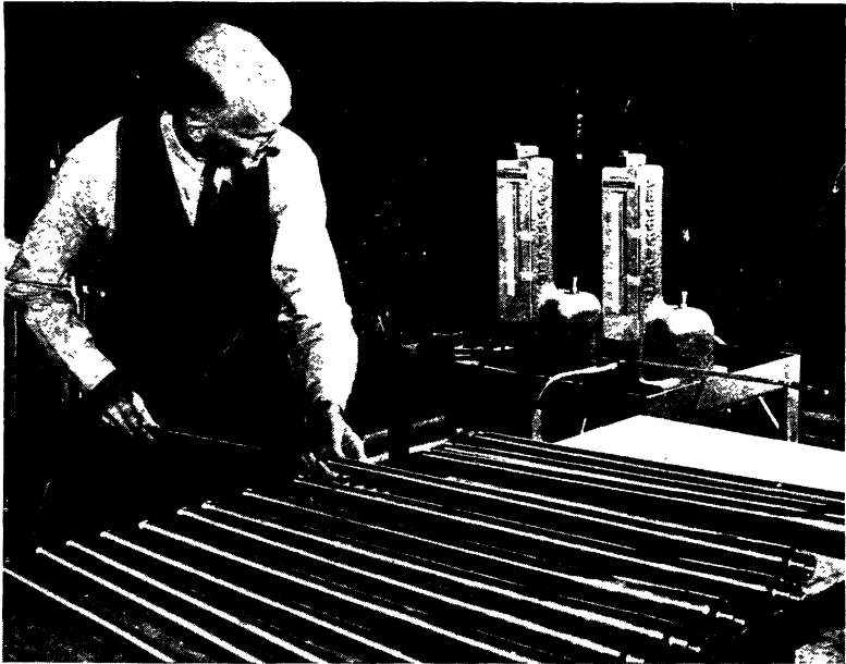
FIG. 88.—Checking gun barrels with air gage.
