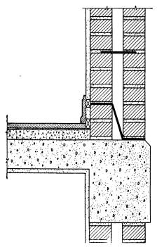
Fig. 130.—Panel wall on concrete skeleton.
