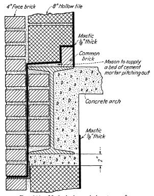
Fig. 144.—Method of spandrel waterproofing.
