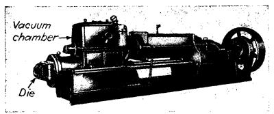
Fig. 37.—Freese improved de-airing machine. It operates successfully in shale, fire clay, and surface clay, producing building brick, firebrick, pavers, drain tile, and hollow ware.
