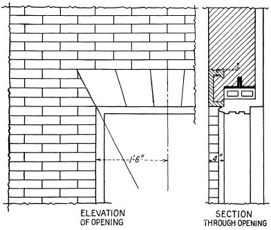
Fig. 142.—Flat arch (brick skewback).
