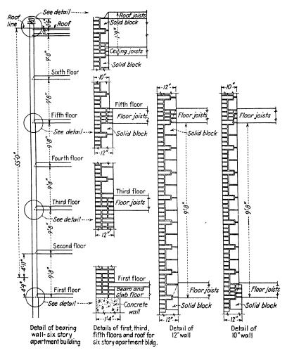
Fig. 103.—Construction details of hollow-masonry (q.v.) wall designed in accordance with the Building Code of New York City, \$C26-431.0.
