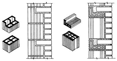
Fig. 108.—Left, Raritile construction, 12-in. combination wall, end-construction tile. Right, header-backer construction, 12-in. combination wall, backer-end construction, header-side construction.
