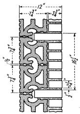
Fig. 107b.—Two Natco Speed-A-Backers,  $7\frac{3}{4}$  in, high with  $\frac{1}{2}$ -in, mortar joints, bond with 6 courses of standard  $2\frac{1}{4}$ -in, brick with  $\frac{1}{2}$ -in, mortar joints. Units  $7\frac{1}{2}$  and  $7\frac{1}{8}$  in, high are available for other mortar joint conditions.
