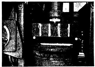
Fig. 11.—Flexural test for bond strength, using a five-brick beam.
