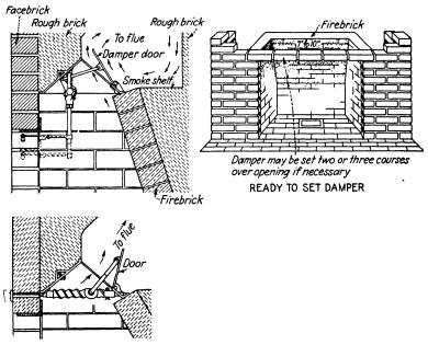
Fig. 149.—Fireplace, with sectional views of damper.
