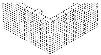
Fig. 25.—4-stretcher Flemish Bond (modified Flemish), return corner.
