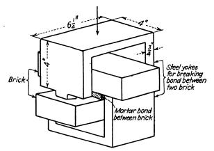
Fig. 9.—Unit of bonded brick in bond-strength device.
