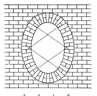
Scale of feet Fig. 74.—Elliptical opening with gauged brickwork.
