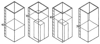
Fig. 33.—Absorption test of brick.
