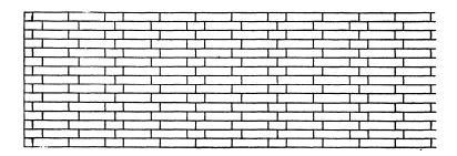
Fig. 24.—4-stretcher Flemish Bond (modified Flemish).
