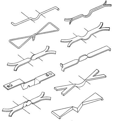
Fig. 129.—Wall ties for cavity wall construction.
