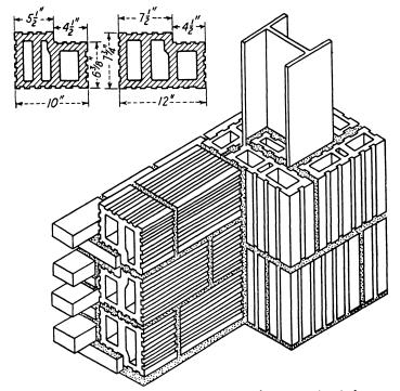
Fig. 105. Unibacker construction and exterior column covering (column covering tile 12 in, high).
