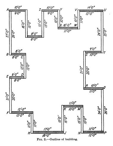
No matter how irregular a building may be, or whether allowance is made for the overlapping of masonry at intersecting corners, the result will never vary more than four corners (4 linear ft. of 12-in. wall).
