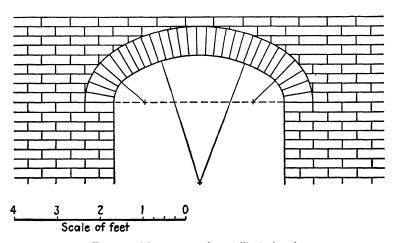
Fig. 63.—Three-centered semielliptical arch.
