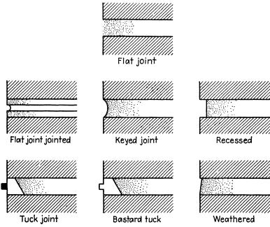
Fig. 18.—Details of mortar joints. (J. Corkhill, "Masonry," London.)
