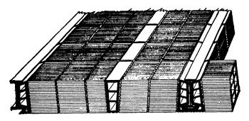
Fig. 121.-Typical combination side- and end-construction arch.
