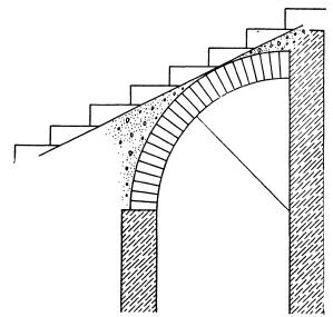
Fig. 67.—Quadrant arch forming soffit of entrance.
