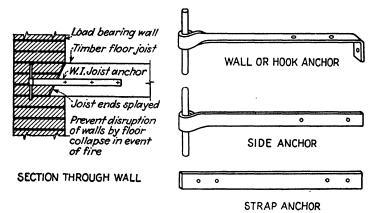
Fig. 1.-Floor joist anchors.
