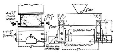
Transverse Brick Testing Apparatus
