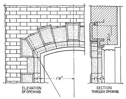
Fig. 141.—Segmental arch (terra cotta skewback).
