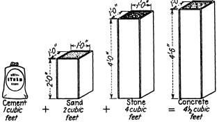
Fig. 4.—Example of 1-2-4 proportion for concrete, showing relative volumes of the three essential materials and the resulting volume of concrete.
