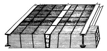
Fig. 120.—Typical end-construction arch (key tiles, side construction).
