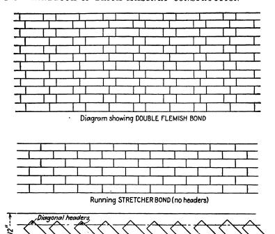
Plan showing running stretcher bond and method of clipping and tieing "CLIPPED" BOND
