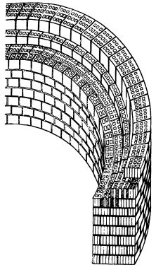
Fig. 150.—Custodis perforated radial brick construction.
