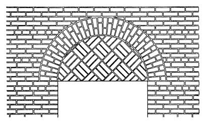
Fig. 53.—Semicircular arch with pattern-filled tympanum.
