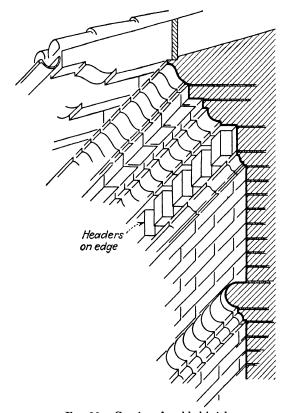
Fig. 96.—Cornice of molded brick.
