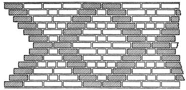
Fig. 43.—Diamond bond (diamond within diamond); 6.76 brick for each square foot.
