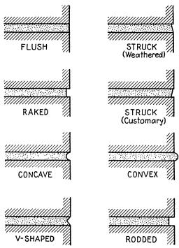
Fig. 13.-Mortar joints.
