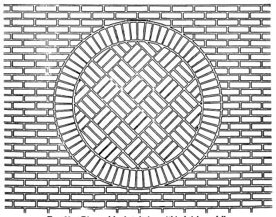
Fig. 69.—Diagonal basket design within brick rondelle.
