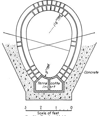
Fig. 75.—Egg-shaped brick sewer.
