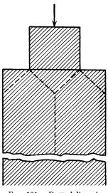
Fig. 101.—Dotted lines indicate lines of likely cracking at failing loads.
