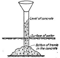
Fig. 3.—Hopper and chute or tremie method.
