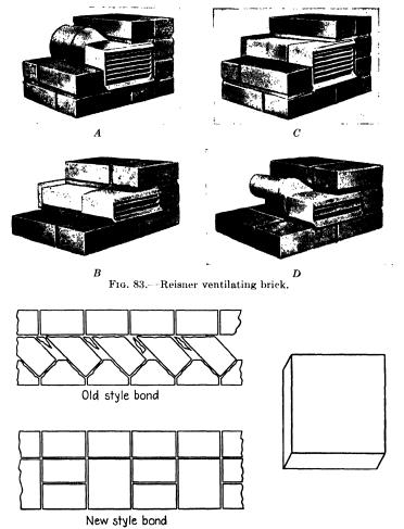
Fig. 84.—Stretcher bond brick. This brick saves labor and the waste of clipping and makes a stronger wall than does the old style of bond.
