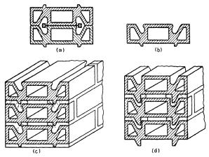
Fig. 77.-Hollow channel brick.
