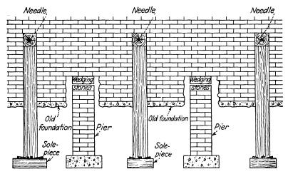
Fig. 145.—Wall of old building supported by needles during the erection of piers extending down to the level of the foundation for the new building.
