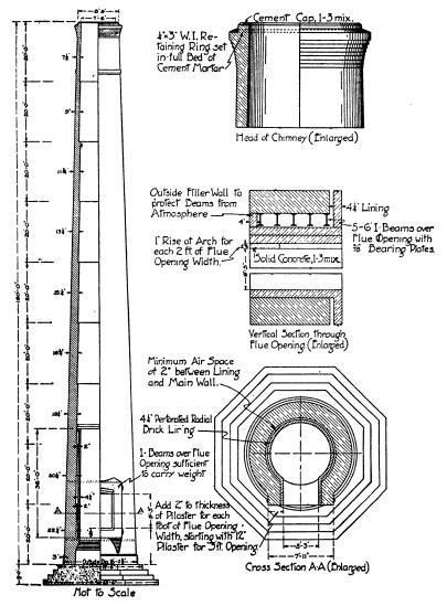
Fig. 151.—Typical chimney, round for the entire height. (M. W. Kellogg Co., Inc.) placed in the brickwork, unless the perforated radial brick have corrugated sides, in which case they may be omitted.
