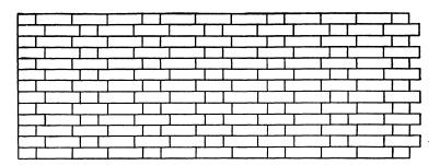
Fig. 22. -3-stretcher Flemish Bond (modified Flemish).
