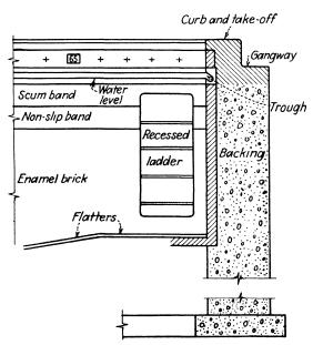
Fig. 156.—Section through pool at low end.
