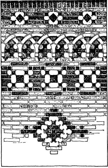
Fig. 50.—Interlaced arches, purpose-made brick. (Architectural Forum, 1917.)
