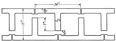
Fig. 127.—Top view of two-piece wall.
