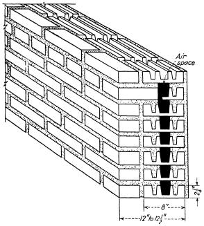
Fig. 82.—Holobond as the backing of face brick in a masonry wall of 12 to 12½ in. thickness.
