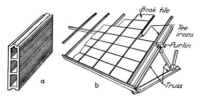
Fig. 125.—a, Standard book tile, square-cut ends. b, Perspective view, book tile in place on structural-steel roof construction.
