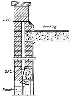
Fig. 132.—Ten-in. cavity wall.
