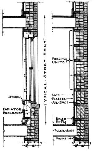
Fig. 119.—Typical wall sections of nonfireproof construction.
