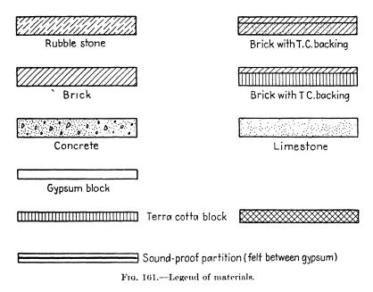
should provide a title for each print furnished. Each plan should have a legend that clearly shows the type of construction and classification of materials. Anything not clear from the drawings should be made so by explanatory notes. The scale of the plan should be given in figures, as, for example, \( \frac{1}{4} \) inch = 1 foot.
