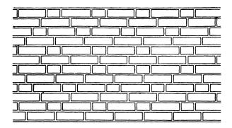
Fig. 29.—Diamond Bond. Diagonal effect obtained by running alternate courses of stretchers and Flemish Bond.
