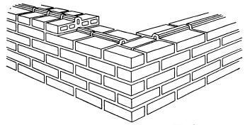
Fig. 79.—Corner of Munlock Drywall brick.
