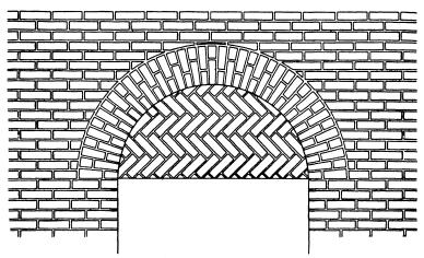
Fig. 54.—Semicircular arch with pattern-filled tympanum.
