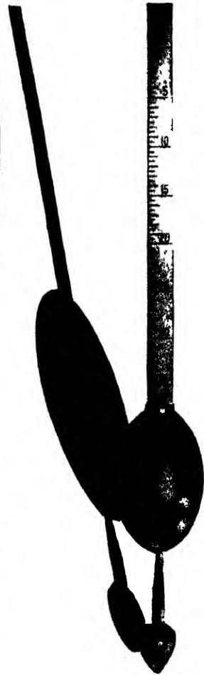
Fig. 59.—Application of the rhodium deposit to metal hydrometers, whereby the latter are rendered highly corrosion-resistant
