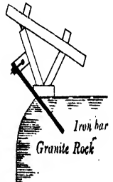
MODE OF SECURING FOOT OF EACH CANTILEVER INTO THE ROCK.
