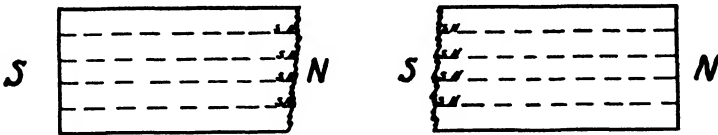
Figure 275 — When a bar magnet is broken, each piece becomes a magnet.
