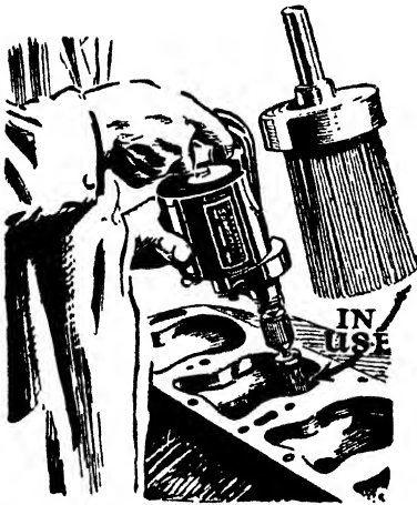
FIG. 47.—Decarbonising Cylinder Head with Wire Brush driven by Portable Electric Drill.
