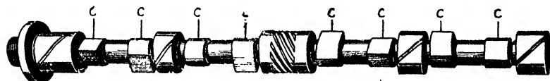
FIG. 97.—Example of Camshaft, showing surfaces at C which can be built up by the Chromium Plating Method.
