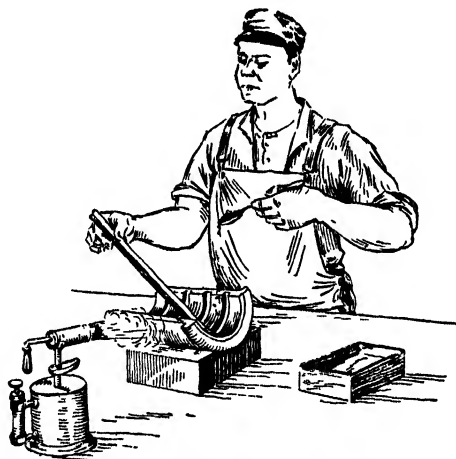
FIG. 114.—Tinning bearing shell before babbitting.
