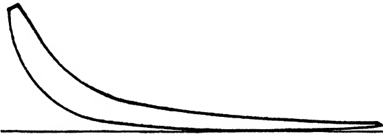
FIG. 218.—Diagram showing high injection-air pressure.
