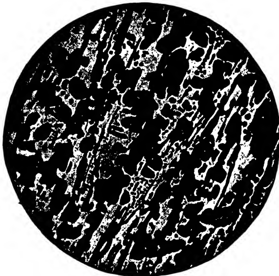
FIG. 34.—White cast iron containing about 3 per cent combined carbon. The light areas are cementite. Magnified 56 diameters. 1
