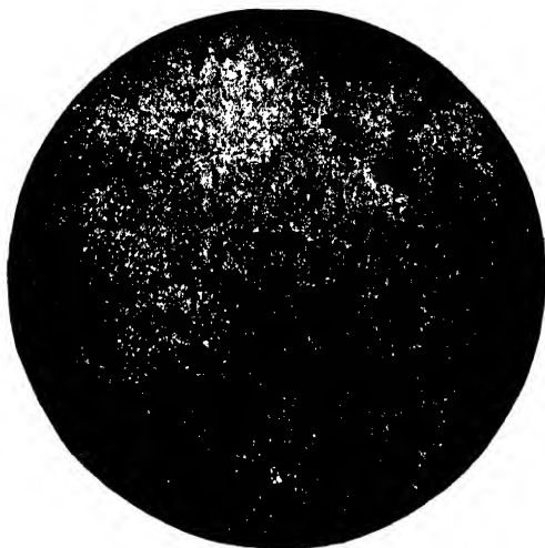
FIG. 61.—Burnt steel. Carbon 1.24 per cent. Magnified 20 diameters. Quenched at a white heat. Unetched. (Osmond.) 1
