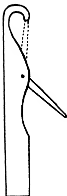
FIG. 71 THE LATCH NEEDLE
