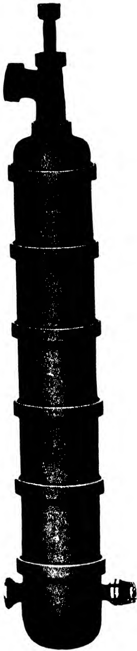
FIG. 103.—“Narki” Metal Denitrating Tower.
