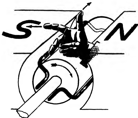
Fig. 32 Fleming's Rule for Generators.
