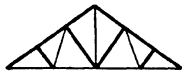
Belgian Truss—2 Panels Less on Bottom than Top—Pitch Fixed by Number of Panels
