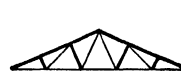
Belgian Truss—1 Panel Less on Bottom than Top—Pitch Fixed by Number of Panels
