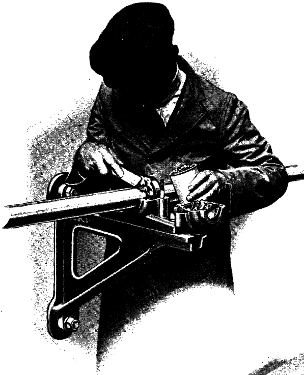
Fig. 19L (Above). —FILL ABOUT \frac{3}{4} OF THE AVAILABLE SPACE IN THE COMPLETE HOUSING WITH BALL-BEARING GREASE
