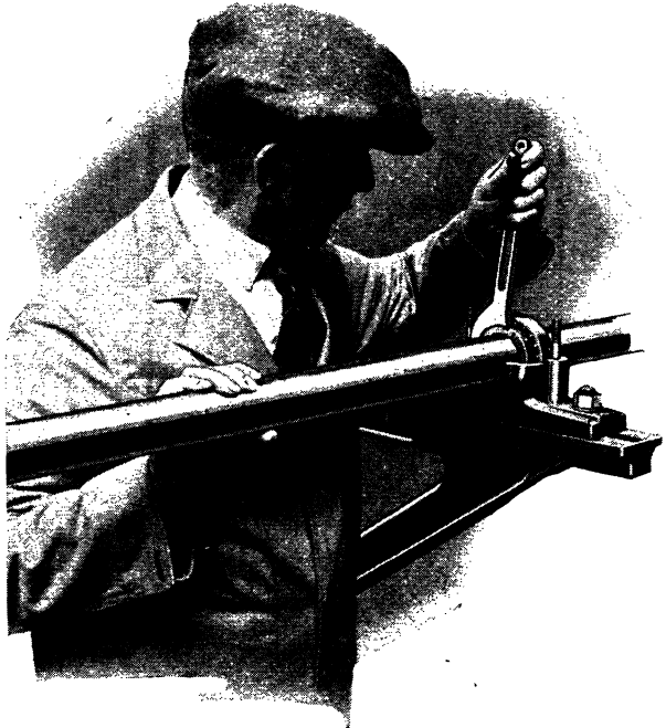
Fig. 19I. —THE BEARINGS ARE SECURED IN THEIR RESPECTIVE POSITIONS BY TIGHTENING THE SLEEVE NUTS
