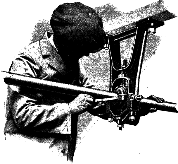
Fig. 19F (Left). —FINALLY EXAMINE SHAFT TO MAKE SURE IT DOES NOT FOUL HOUSING AT ANY POINT
