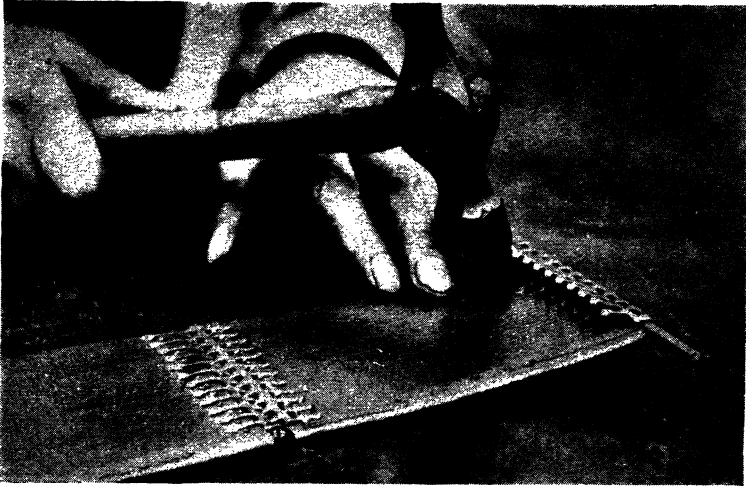
Fig. 10. —ALLIGATOR-TYPE FASTENER BEING DRIVEN HOME
