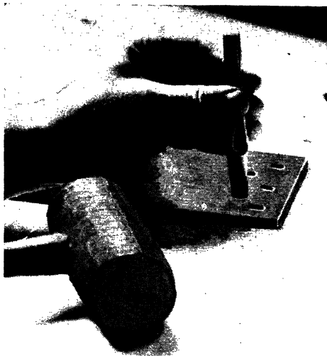
Fig. 8.—PUNCHING LEATHER BELTS FOR LEATHER LACING
