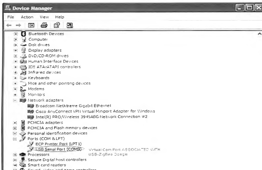
Figure 5-5: USB-ZigBee Dongle associated with a COM port
