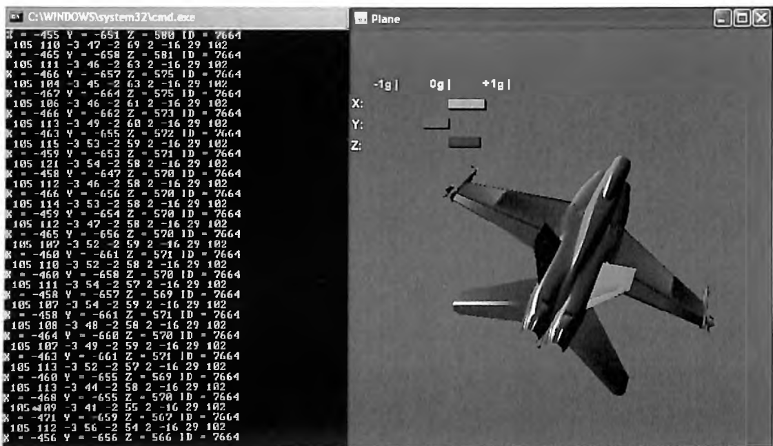
Figure 5-9: Object orientation controlled by ZigBee using MEMS
