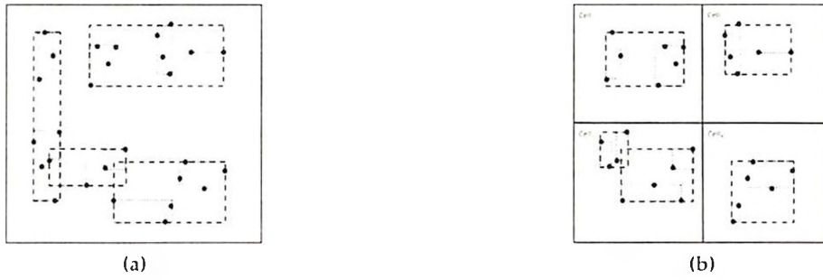
Figure 2.2: Illustrating MBRs formed over a two dimensional synthetic dataset using (a) R-tree (b) Grid-R-tree
