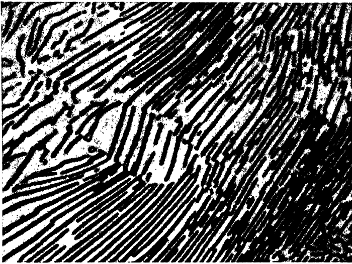
FIG. 3.6. Coarse pearlite formed at 1300°F. (705°C.). 2000 \times . ( Forgeng. )
