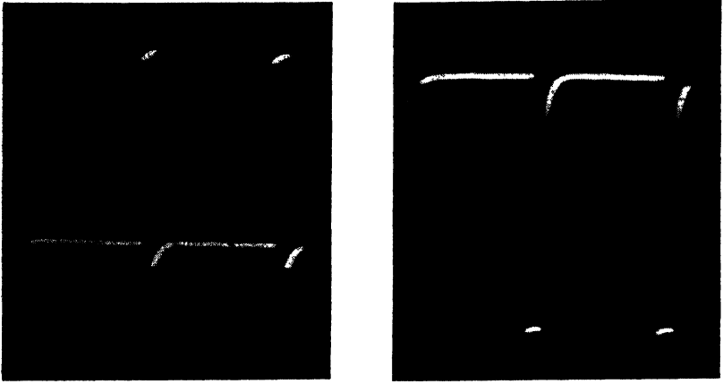
Fig. 2.39. Cathode-coupled multivibrator, plate-to-ground voltage ( E_{p1} ). Shows the total range of gate width available by adjustment of the voltage E_{p1} .
