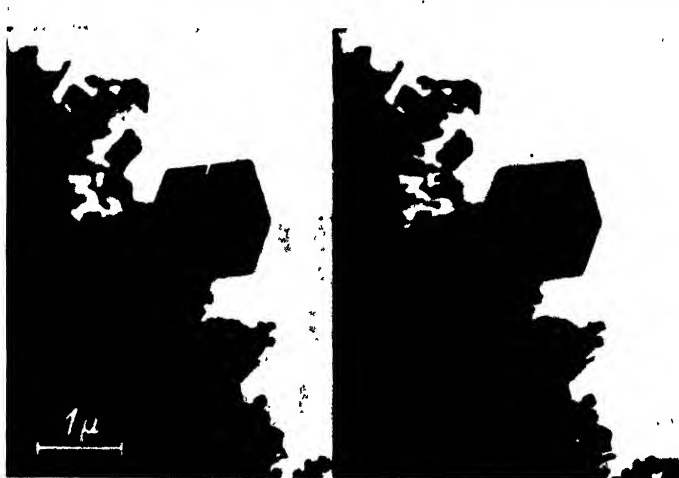
FIGURE 14. Micrographs of magnesium-oxide smoke obtained with the electrostatic electron microscope: (left) with the electron beam potential varying over a range of 50,000 volts; (right) with a filtered beam potential. This comparison shows the insensitivity of the electrostatic electron microscope to fluctuations in the accelerating potential of the illuminating electron beam. 105
