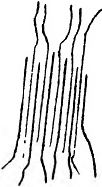
F. Fringed micells according to the new theory (after Kratky).
