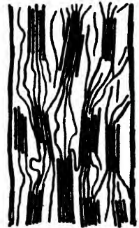
H. Behavior of cellulose chains in a rayon spinning solution, coagulated and oriented (after Mark).
