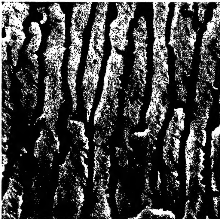
FIGURE 33. Replica of Pearlite structure prepared by double replica process of Heidenreich and Peck. 76 Opaque areas represent elevations; transparent areas represent depressions in original sample. (Courtesy Dow Chemical Co.)
