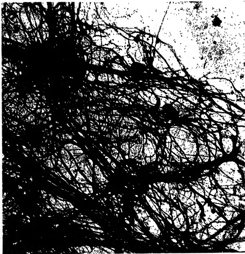
FIGURE 28. Fifteen-day cotton fiber (X 8000) partially disintegrated. Two phases can be seen—a very dense material which is almost completely opaque to electrons, and an extremely fibrous material. 30 (Courtesy American Cyanamid Co.)
