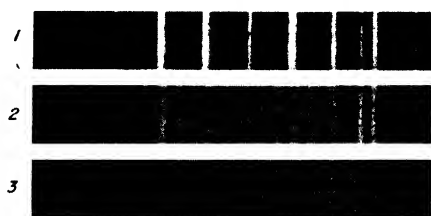
Fig. 71. Transformation of a resonance spectrum of I_2 to the complete band spectrum (Franck and Wood).
