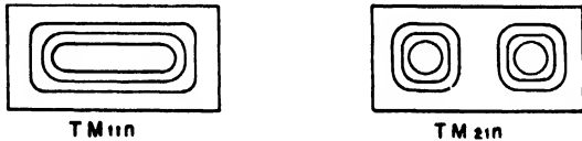
FIG. 5.36 Configurations of the magnetic field for transverse magnetic modes.
