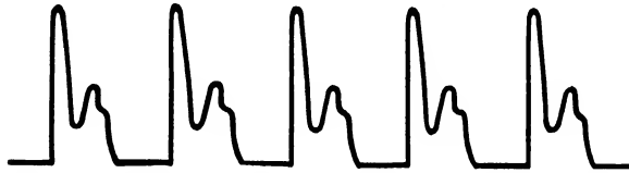
Fig. 12-54 Oscillogram of shunt-tuned input current. (From Electronic Transformers and Circuits by Reuben Lee.)
