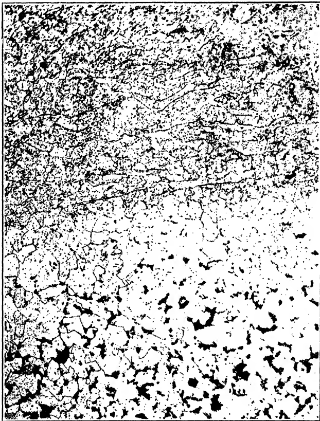
*FIG. 29.—Same as fig. 28, but after heat treatment at 900° C. for one hour. Etched. \times 150 .
