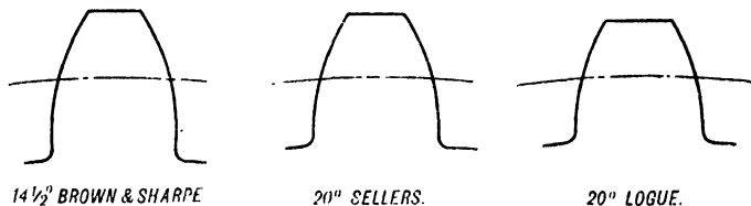
FIG. 5.—Forms of Gear Teeth.
